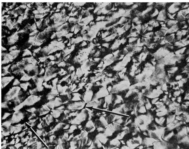
Fig. 6. Effect of pressurization on microstructure; (a) bright-field light (40 \times ); (b) cross-polarized light (200 \times ).
