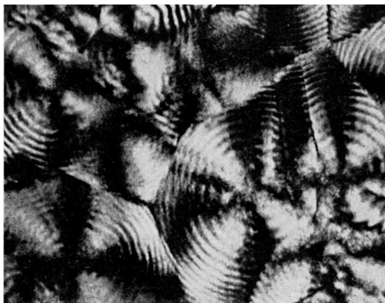
Fig. 10. Spherulitic texture of linear polyethylenes ( a ) of melt index 0.2 (200 \times ); ( b ) of melt index 3.6 (200 \times ).
